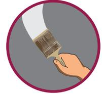
Apply 1 or 2 coats of Berger Bio-Wash solution (5%v/v) and allow it to dry overnight.
