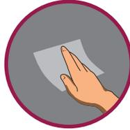
For fresh/new surfaces: Strip all loose particles from the surface with wire brushing and by scraping, followed by a wipe down. Wash the surface down with water and allow it to dry.
